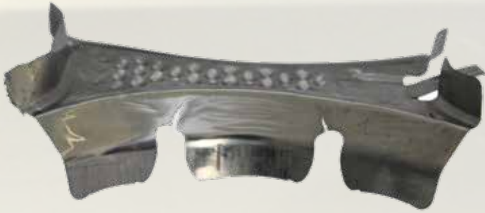
Heat shield with folds and cracks confirms simulation result
