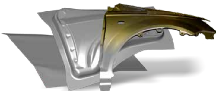
Stampack Trim Optimizer saves costly laser-cut prototypes and thus also valuable trial and development time.
