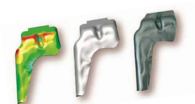
3D volume simulation allows the exact simulation of the forming process: reality (right) and simulation (center) are practically indistinguishable.
